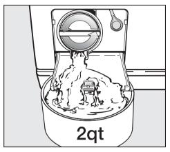
■ Turn the lint trap lid counterclockwise. Do not remove it. About 2 quarts (2 liters) of water will drain out of the hose.
