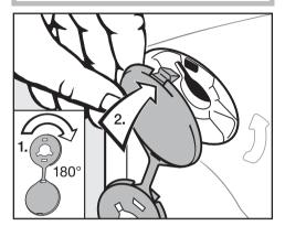
■ Close the holes with the rotary protectors as shown, making sure to close the caps.
