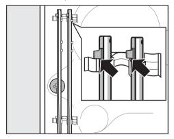
■ Fasten the shipping struts to the rear of the washer. Make sure that the catch at the top of the strut is hooked above the holder.
