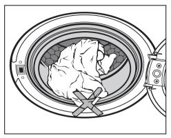
To prevent damage to the door seal and clothing, make sure that there are no clothes caught between the drum door and the seal.
