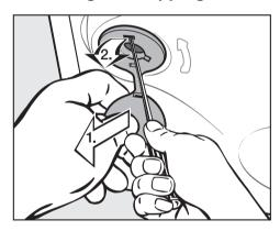
■ Remove the left and right rotary protectors. Pull, 1, the attached rotary protector, then use a screw driver to release, 2, the catch at the top.
