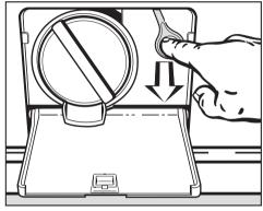
■ To open the door, pull down on the ring in the upper right corner of the access area.
