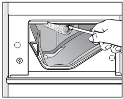
■ Using a bottle brush remove any detergent or lime deposits from the water inlet valves at the top of the detergent drawer niche.
